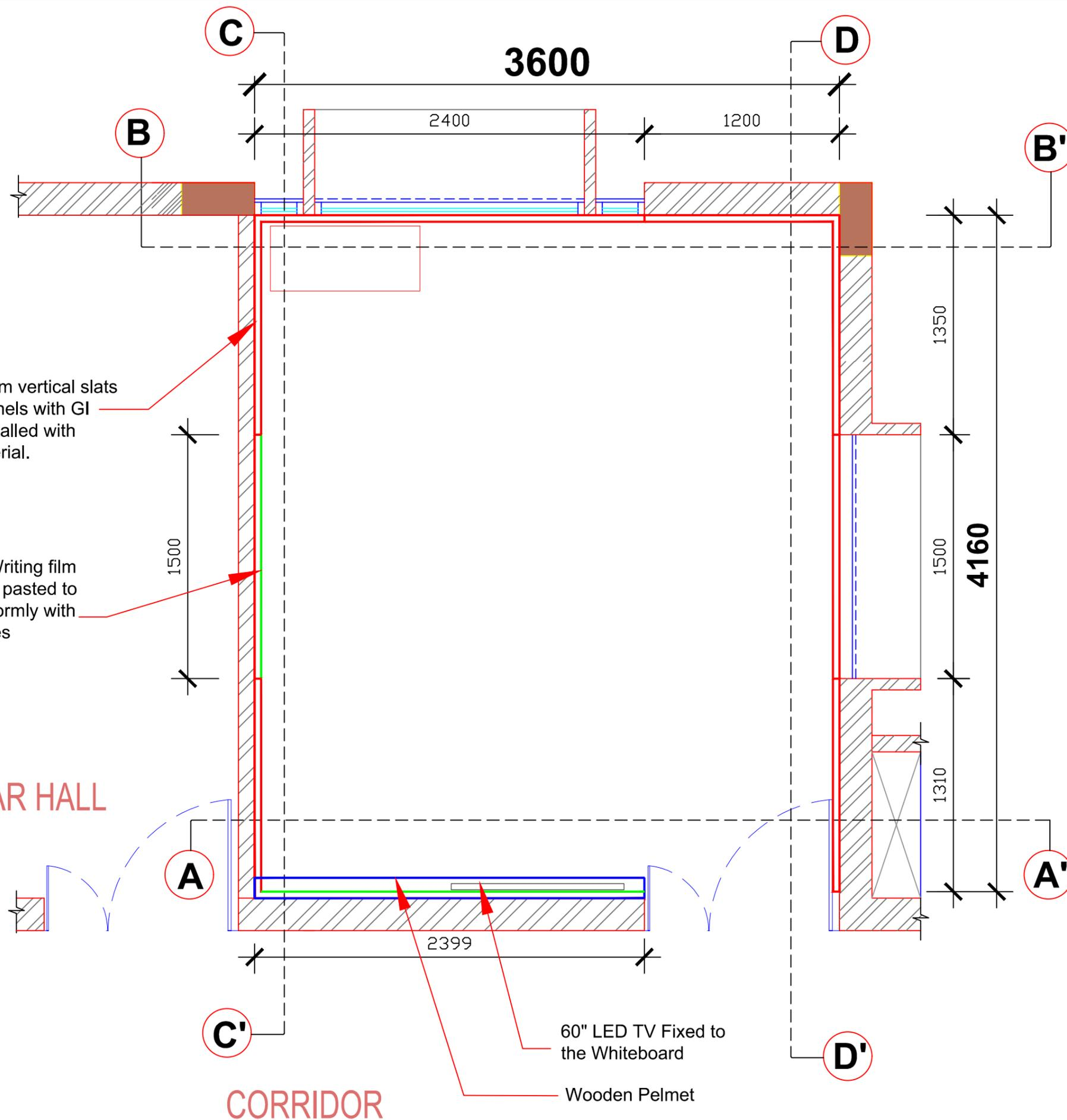
Anutone 16mm vertical slats acoustical panels with GI support & installed with acoustic material.
